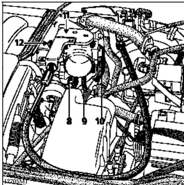
Completely remove the engine tie bar.
