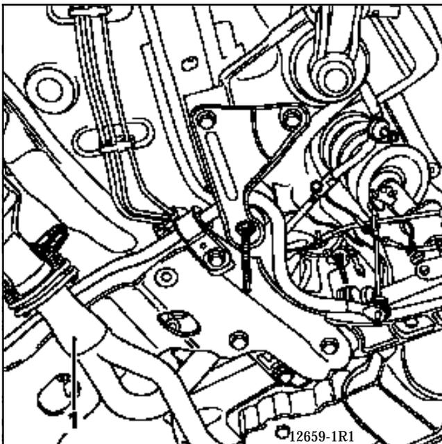
Remove the engine tie bar and push the engine slightly forwards (be careful not to interfere with the cooling radiator). Insert a shim between the sub-frame and the gearbox.
