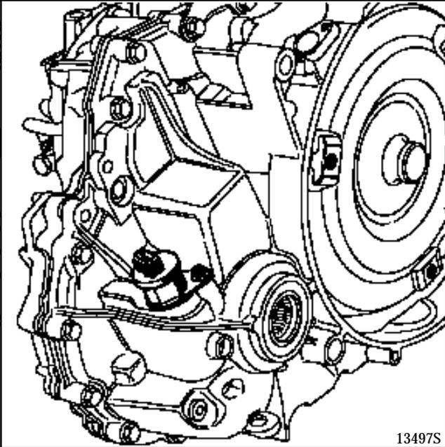
Replace the speed sensor pin if necessary.
