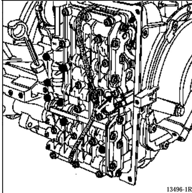
Move the distributor to one side and remove the output speed sensor mounting bolt.
