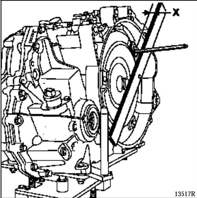
Use a trammel (P) to make it easier to position the converter.
