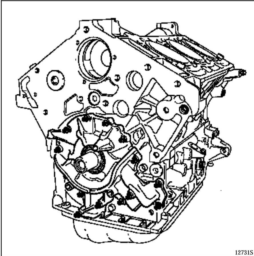
**NOTE:** the sealing of the oil pump is ensured by a composite seal which can endure several removal operations. If the seal is damaged, it can be partially repaired using the sealing product **AUTOJOINT OR**.
