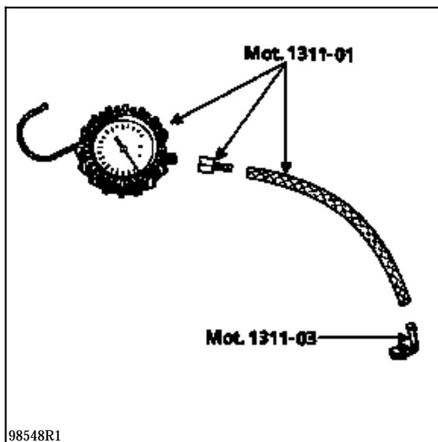
Shunt the terminals of the pump relay (A) in the engine connection unit. Check the pressure. It should be  $3 \pm 0.2$  bars.
