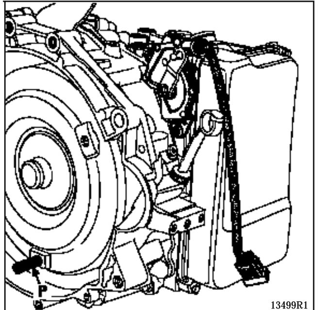
**DO NOT USE ANY BOLTS OTHER THAN THE ORIGINAL BOLTS PROVIDED FOR FITTING THE CONVERTER TO THE STARTER PLATE**
