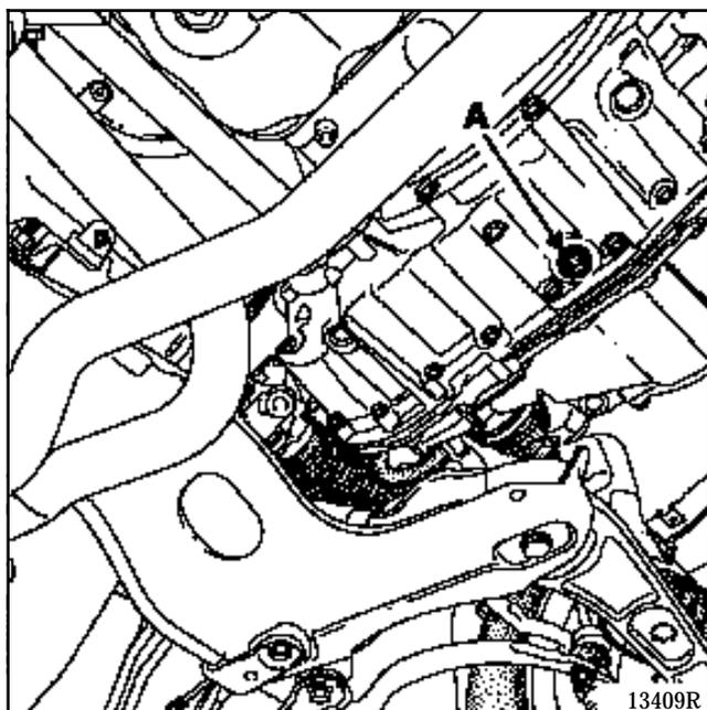
Remove the faulty differential output seal using a screwdriver or a hook, taking care not to scratch the contact surfaces.
