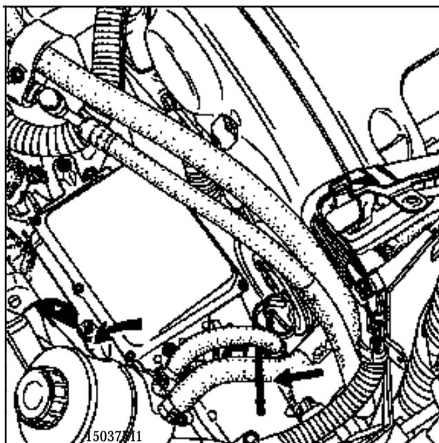
Slacken the power assisted steering pump unions.
