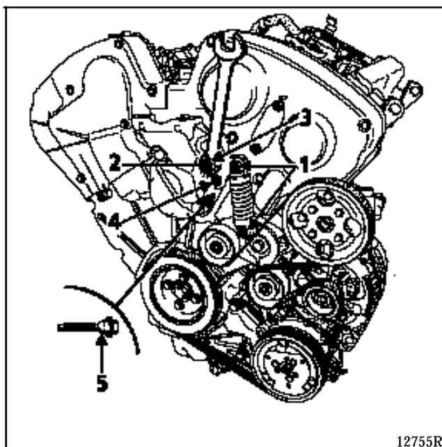
When refitting, place the dynamic tensioner in the operating position towards the right and tighten bolts (4) then (2) to a torque of **2.5 daN.m**.
