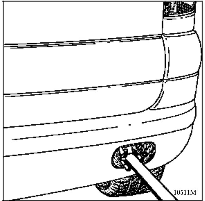
Remove the ring cover from the left of the front right hand additional headlight or the rear cover on the right hand side of the bumper and fit the shackle into the ring.
