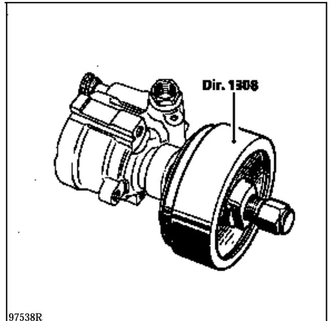
Use an extractor (releasing tool) to remove the hub and push on the pump shaft with a press.
