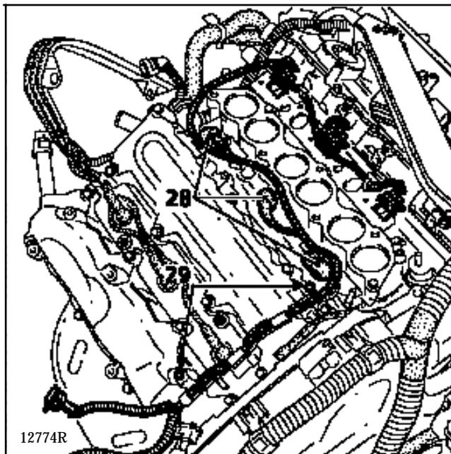
Remove the inlet distributor mounting bolts.
