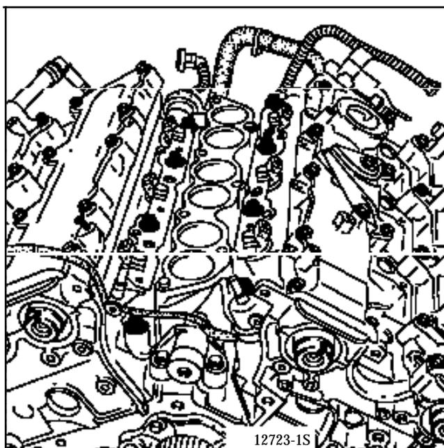
Remove the distributor and the injector galleries.
