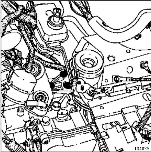
Raise the vehicle in relation to the engine and transmission assembly (operation requires two people).
