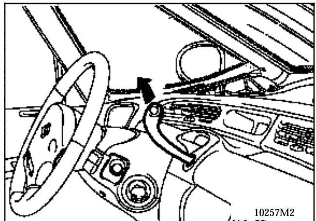
Check that the lever moves between the various positions correctly ("gears").
