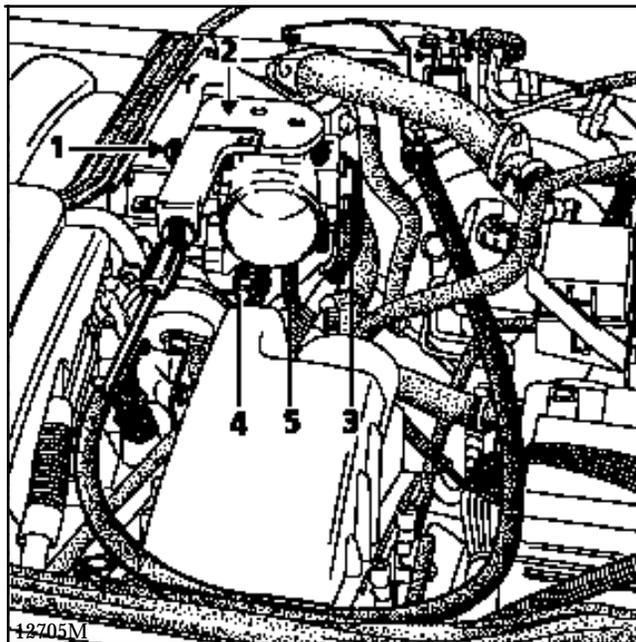
Remove the throttle body mounting bolts then remove the throttle body.
