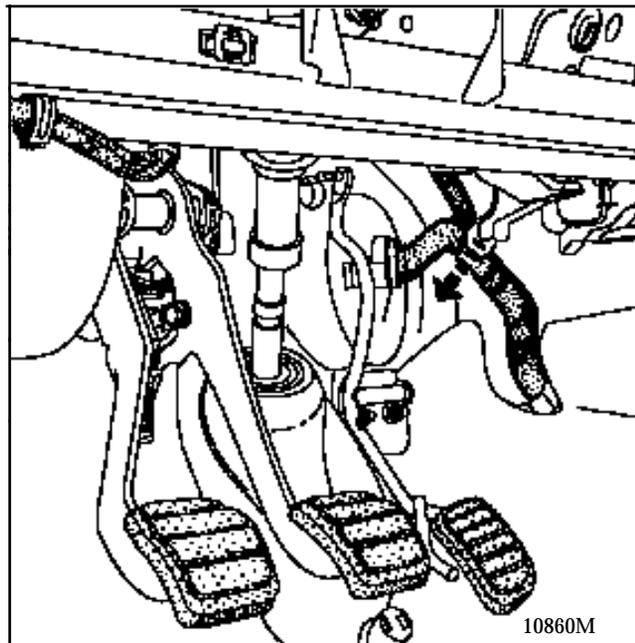
Check that there is no interference between the passenger compartment wiring loom and the lower left hand angle of the storage tray.
