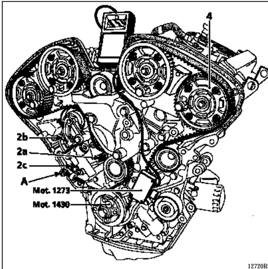
Tighten bolt (A) until you obtain a tension of **83±2 SEEM units**.
