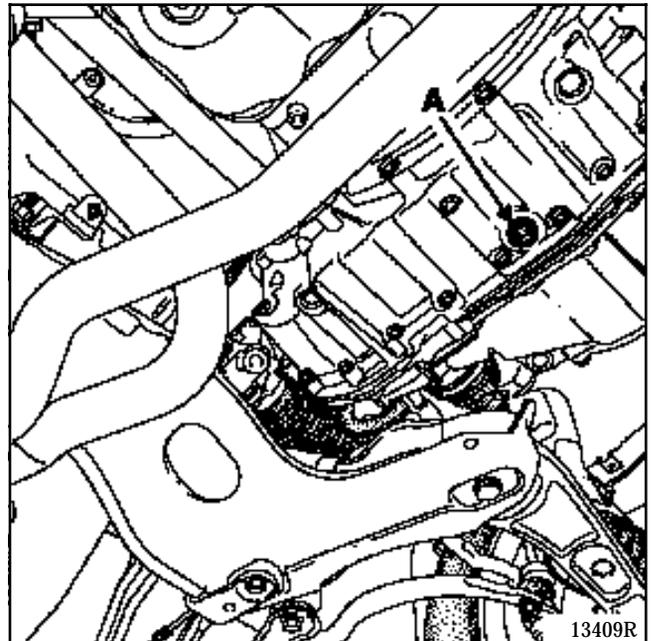
Measure the quantity of oil drained (this measurement is used as a reference for refilling).
