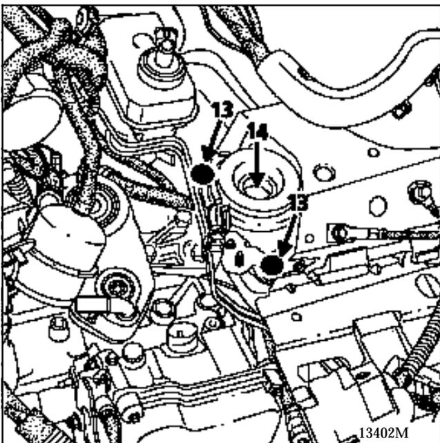
Remove the right hand suspended engine mounting cover.
