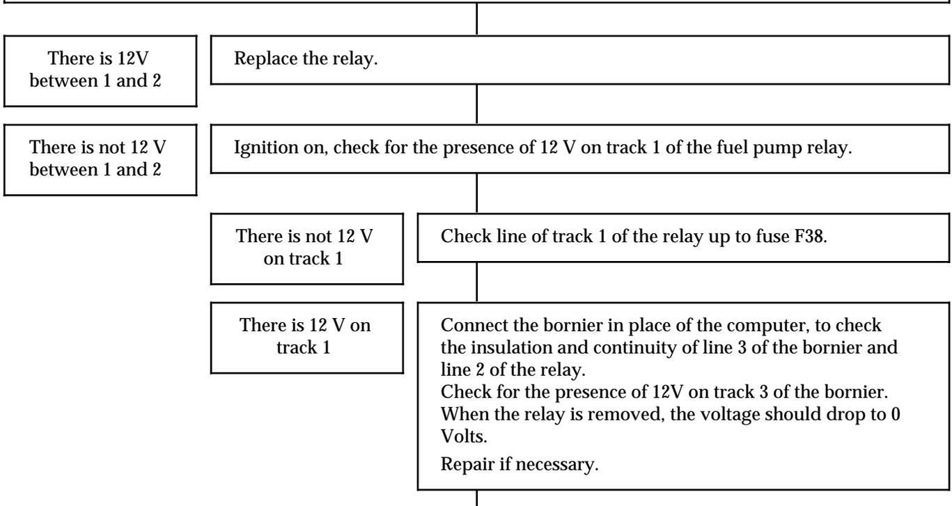
The problem is still not resolved! The injection computer must therefore be replaced.
