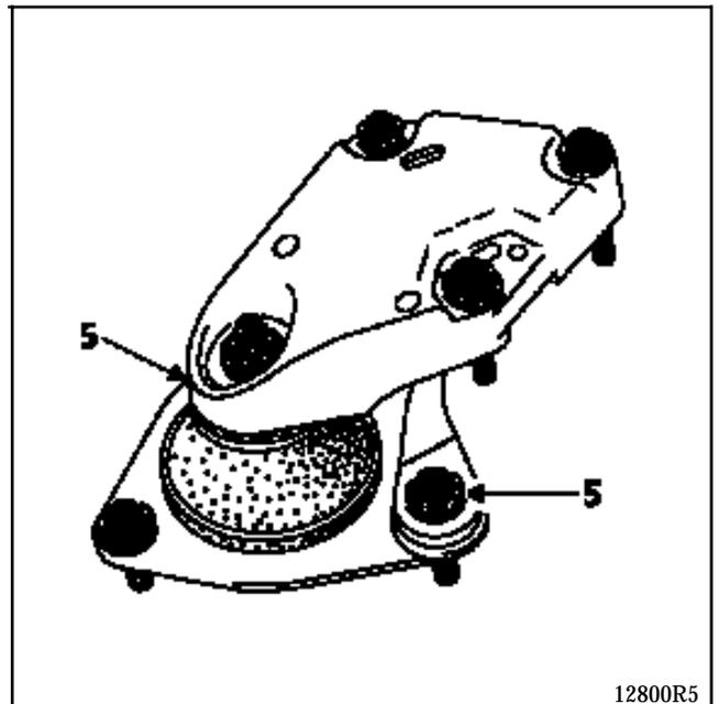
Tighten the limiter bolts (5) to a torque of **6.2 daN.m.**
