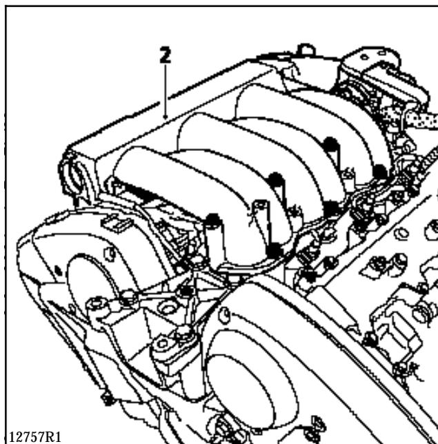
To remove the plugs, use the plug kit, **Ele 1382**.
