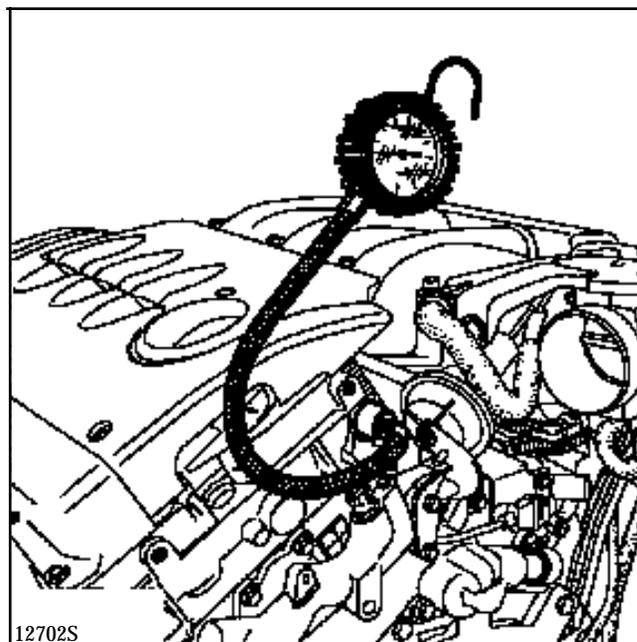
By applying a vacuum of 500 mbars to the pressure regulator, the fuel pressure should be  $2.5 \text{ bars} \pm 0.2$ .
