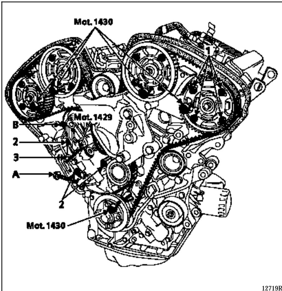
Turn the camshaft sprockets clockwise until they lock into the slots.
