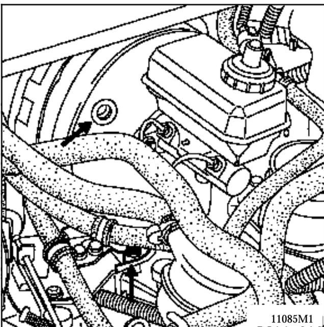
Unhook the wiring loom from the brake servo mounting to allow the cable to pass through.
