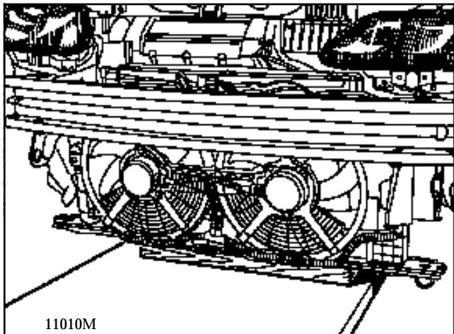
Remove the two cross member mounting bolts on the side members and raise the vehicle to remove the cooling assembly.
