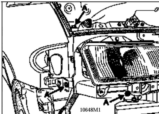
Remove the power assisted steering oil reservoir from its mounting and place it to one side.
