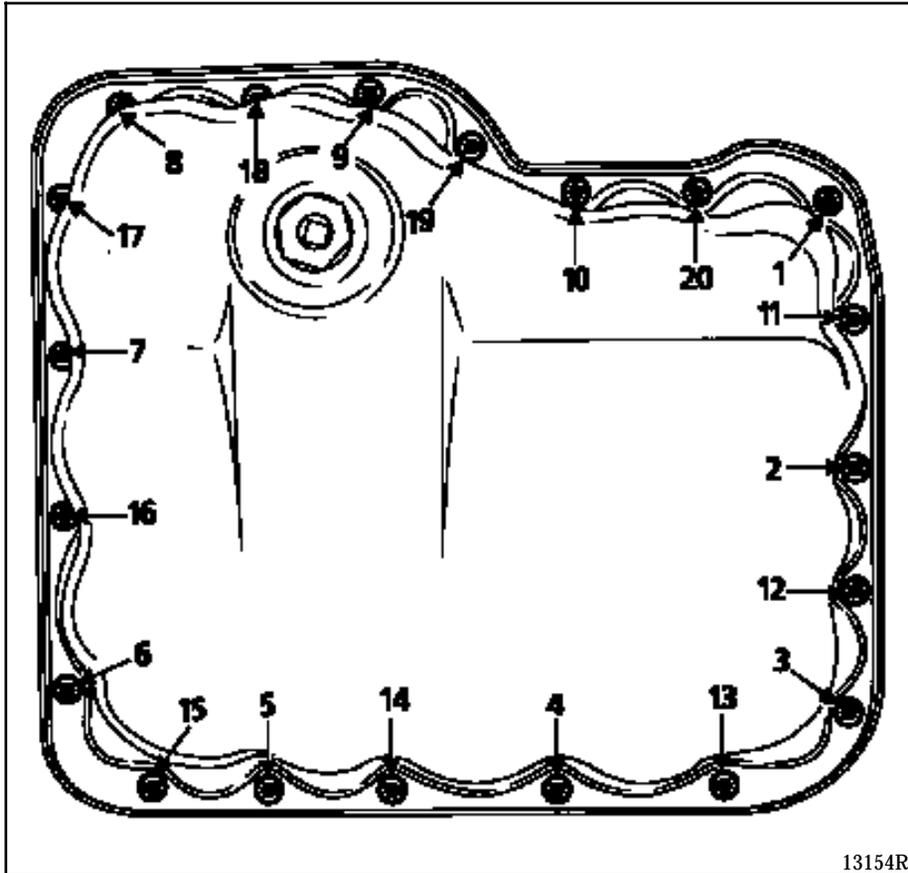
**NOTE:** the sealing of the sump is ensured by a composite seal which can endure several removal operations. If the seal is damaged, it can be partially repaired with the sealing product **AUTOJOINT OR**.
