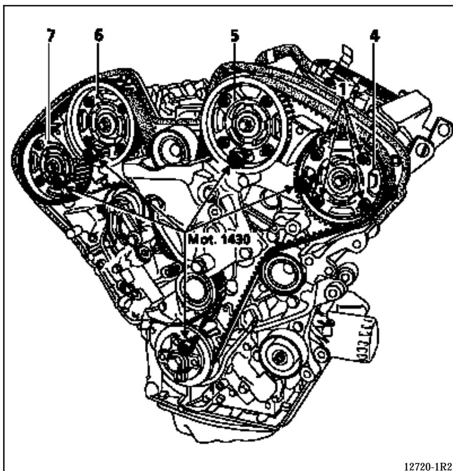
Tighten bolts (1) to a torque of **1 daN.m** starting from sprocket (4), then (5), (6) and (7).
